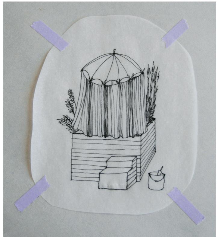
**3** Next, assemble a platform with a hole for the toilet seat. Secure it on the front (long) edge of the planter. Put a cardboard box directly below the toilet seat.
